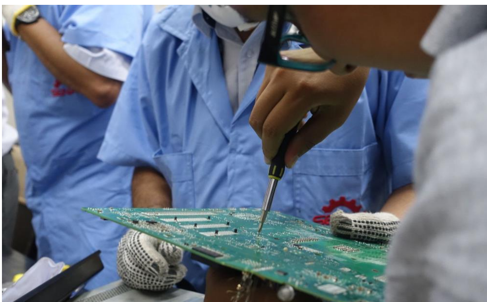
Figure 1. Disassembly of a PCB board (Source: SRI)
