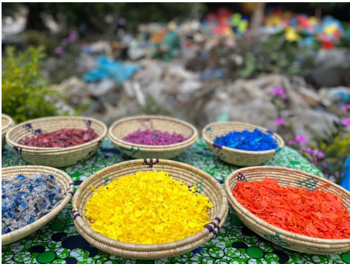
Figure 3. Shredded plastic segmented by colour (Source: SRI)
